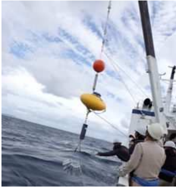
Bottom mooring ADCP
