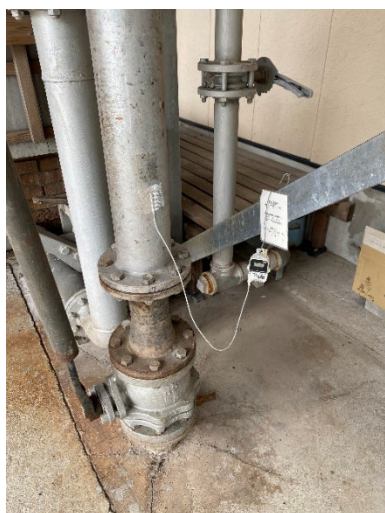
Continuous measurement of hot spring source temperature (Obama Onsen)
