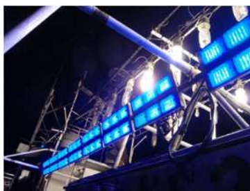
LED lights installed on squid fishing boats
