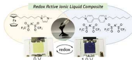
Figure 3. An electrochromic device constructed by a mixture of ferroceneion and viologen ionic liquids.
